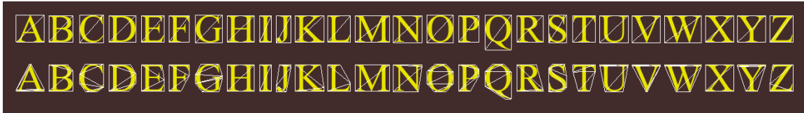
Figure 4. To reduce the number of pixels rendered for most glyphs, simple quads are replaced with polygons having up to eight sides after the corners of the bounding boxes are clipped.
