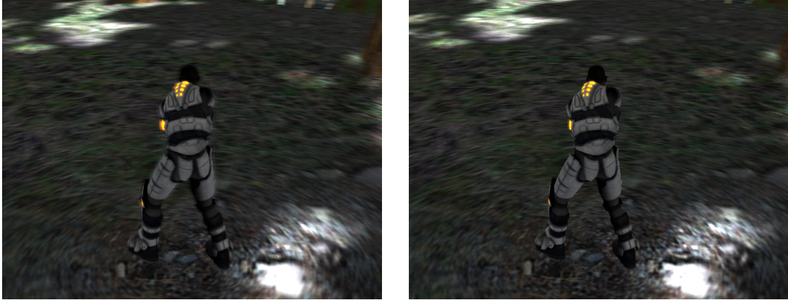
Figure 3. In these two images, the camera is rotating around the character, causing the ground to move across the screen while the character is almost completely still. In the left image, the depth and gradient information in the velocity buffer is not considered, and all color samples along the direction of the velocity are used. Notice the ghosting of the glowing parts of the character's armor and the fuzzy halo surrounding his legs. In the right image, the depth and gradient information in the velocity buffer is considered, and the rejection of the appropriate color samples eliminates the artifacts.
