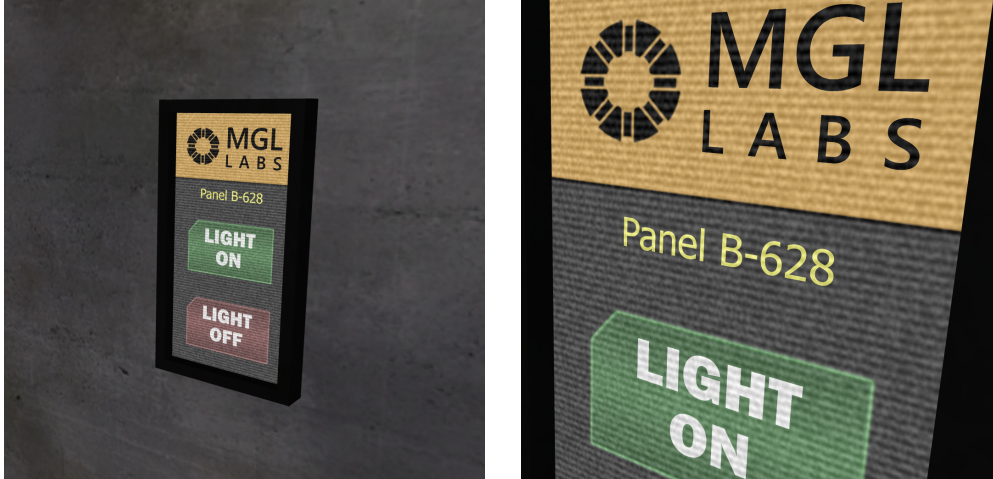
Figure 1. Glyphs are rendered in a game level directly from Bézier curve data extracted from a TrueType font. Because no precomputed images or distance fields are utilized, the results are pixel accurate under any affine or projective transformation, including all scales, rotations, and perspective distortions.
